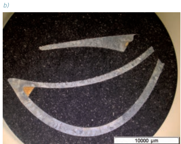
Figure 2. Grain structure predicted by the modelling tool (a) and optical microscopy image of the grain structure in the solid vane of the NGV (b). The dashed line on (a) marks the cut plane on (b). The location of the analysed section is marked by the red circle on the NGV icon (a).
