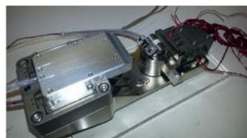
Figure 2. (a) Micropillars machined by FIB on the surface of a wrought Inconel 718 alloy. (b) Deformed pillar on the  $\langle 012 \rangle$  orientation showing the activation of different slip systems. (c) In-situ micromechanical stage to carry out tests in the SEM at temperatures up to 800°C.
