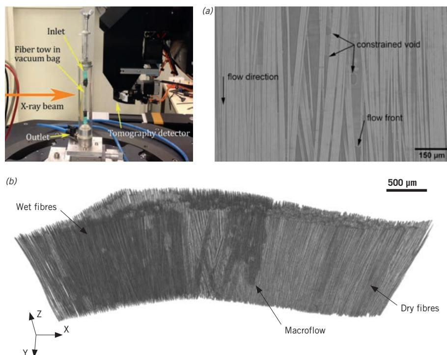
Figure 5: Set-up of the infiltration device. a) Longitudinal cross section of the impregnated tow showing trapped voids and the flow front meniscus. Local fiber misalignments with convergent/divergent trajectories are also visible. b) 3D rendering of fiber tow showing dry and impregnated regions.
