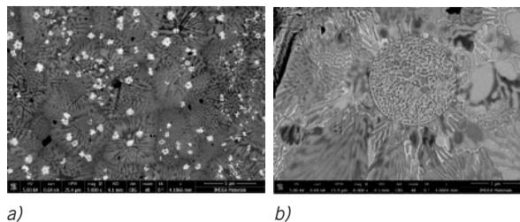
Figure 2. Microstructure of the powder alloys atomized for ALM (a) Ti-29Fe-9Sn-5Nb and (b) Fe-15.5Ti in wt%. The eutectic microstructure is revealed by FEG-SEM.
