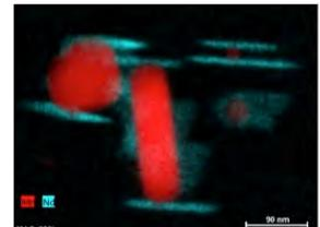
3D-EDS: precipitates in a Mg-Nd alloy
