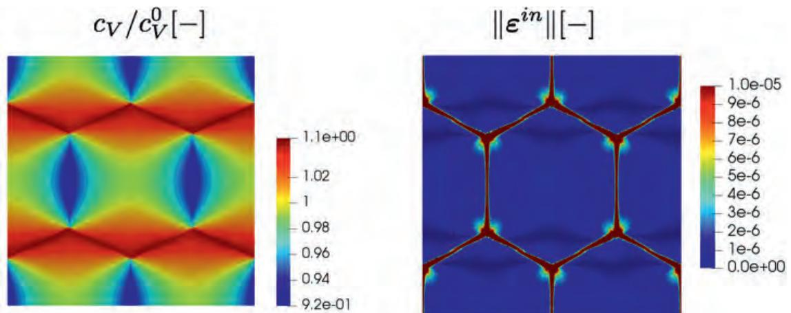
Figure 1. Diffusional creep simulation in a 2D polycrystal (a) vacancy distribution (b) inelastic deformation due to vacancy flux.
