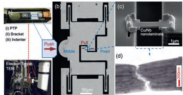
Figure 1. (a) Scheme of the experiment set up (b) Push-to-pull device to carry out in-situ tensile test in the TEM, (c) Electron transparent specimen, (d) Final fracture of the specimen.
