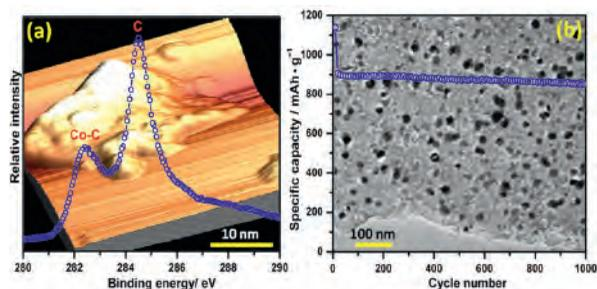
Figure 3. (a) AFM image / C 1s XPS spectra and (b) TEM image/ electrochemical performance of cobalt nanoparticles chemically bonded to porous carbon nanosheets.
