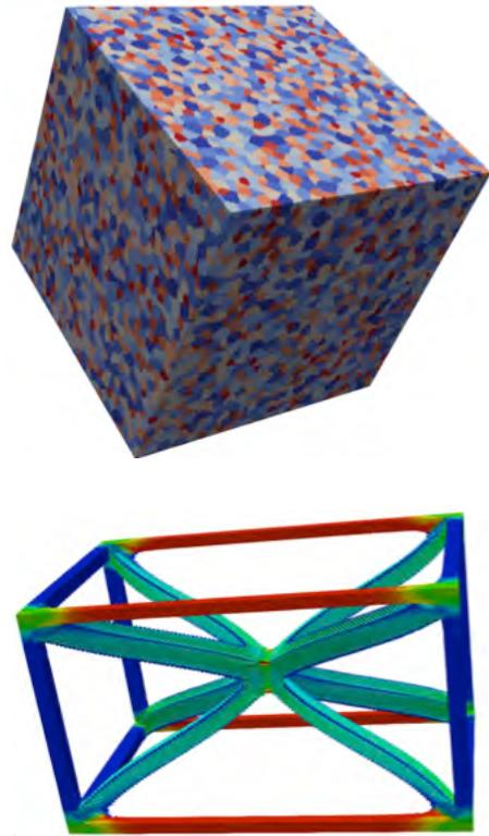
Figure 1. Up: Polycrystalline model containing 120.000 grains and  $16 \cdot 10^6$  voxels. Down: Deformation of lattice structure,  $2 \cdot 10^6$  voxels
