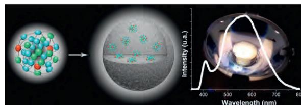
Figure 4. Left. Sketch of white-emitting silica nanoparticles consisting of a core made of blue, green, and red emitters and a silica shell. Right. Picture of a hybrid LED, in which the UV-chip (390 nm) is covered by a color filter with white silica nanoparticles that transform the UV light into sun-like white as shown in the electroluminescence spectrum.
