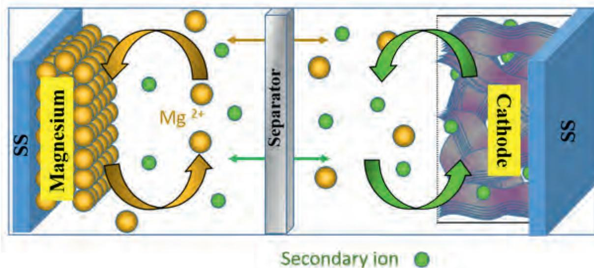
Figure 1. Schematic for Mg hybrid: The magnesium metal perform as the anode where as specially chosen material with specified morphology would perform as the cathode. The charge storage at the anode is dominated by the  $\text{Mg}^{2+}$  ions however at the cathode the secondary hybrid ion dominates.
