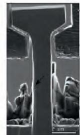
Micropillar compression / microtensile testing in SEM/TEM
