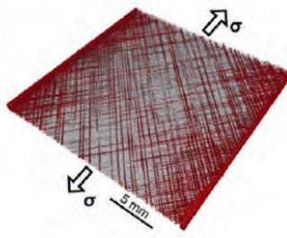
Composite failure in XCT
