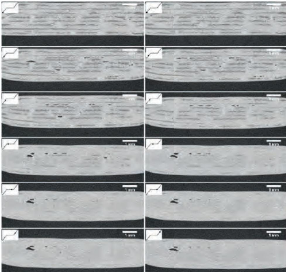
Figure 4. Time sequence as obtained from XCT in the same slice during the curing process of an Out-of-Autoclave composite material. The inset indicates the curing conditions (temperature and time).
