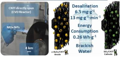
The remarkable efficiency obtained is due to the morphology of the electrodes, in which the CNT fibres act simultaneously as a current collector, active material and support for the metal oxide. Such architecture leads to high capacitance while minimizing internal resistance.
