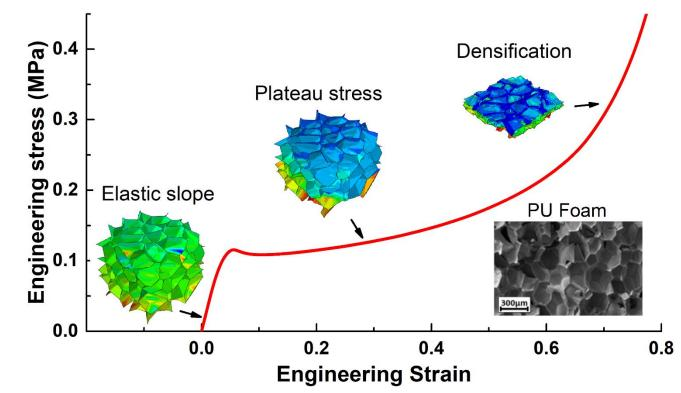
Simulation of the mechanical response of a closed-cell polyurethane foam in compression. The model takes into account the influence of the gas pressure within the cells and of the contact between struts during crushing.
