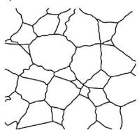
Central cross-section of the representative volume element showing the deformation of the cell walls. (a) Initial cell wall structure. (b) Cell wall structure after 6% compressive strain.
