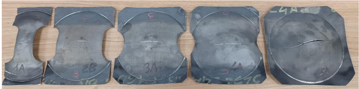
Figure 5-23. Typical appearance of tested Nakajima samples.
