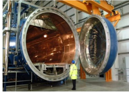
(a) An autoclave.
