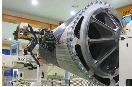
(c) Automated fibre Placement AFP.
