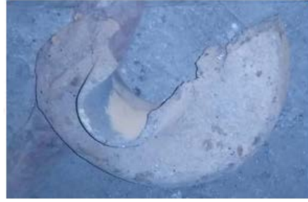
Figure 3.3: Example of the damage of a gas injection nozzle [9].
