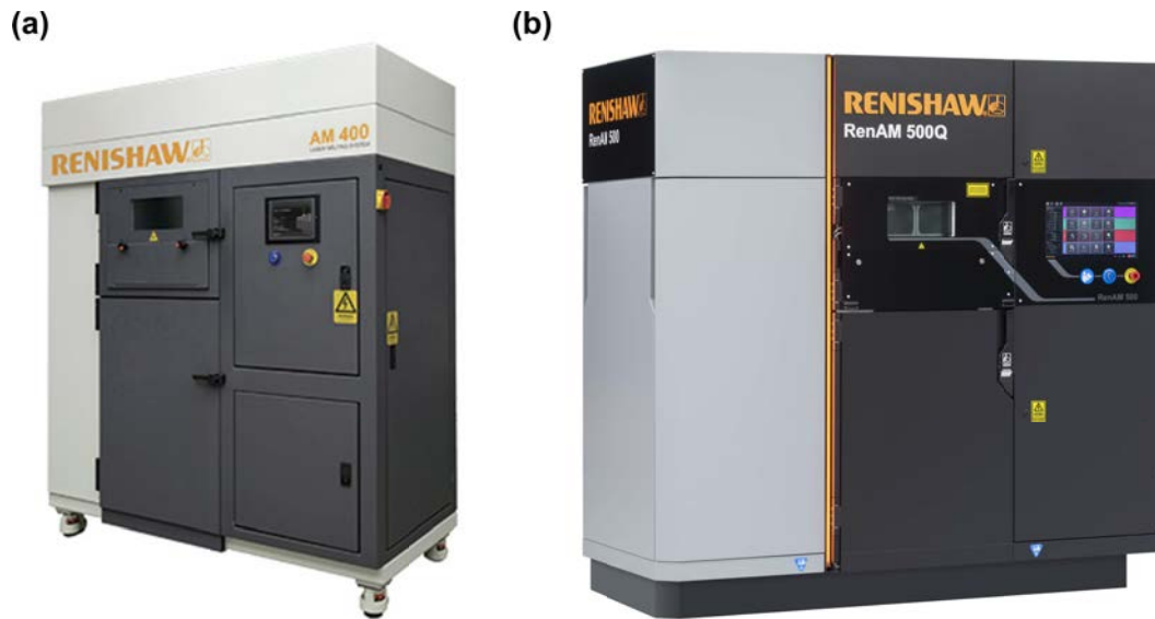
Figure 3.2. Laser powder bed fusion systems used in this work. (a) AM400; (b) RenAM500Q.
