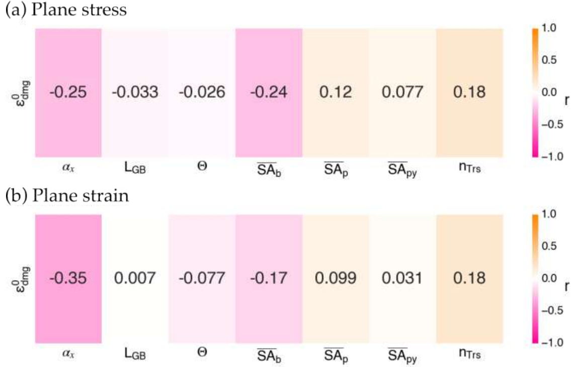
Figure 7.16: Pearson correlation matrix for GB fracture in the Mg foils with random crystal orientations. (a) Plane stress, (b) plane strain.
