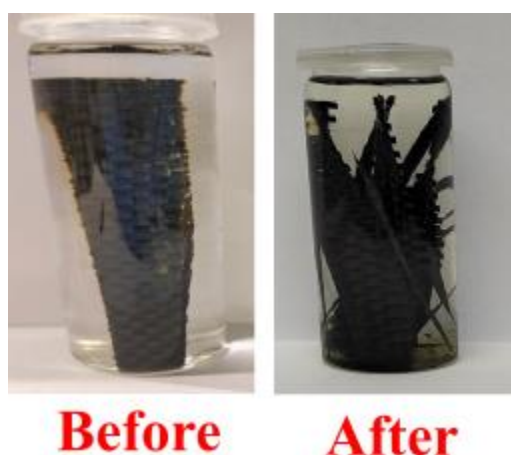
Figure 5-9 Photographs of the GTV-4-CF polymer before and after degradation in EDA solution.
