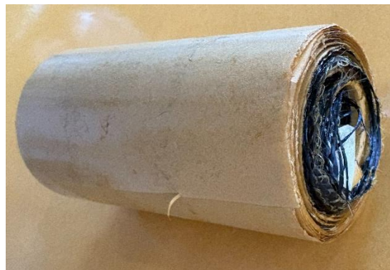
Figure 6-3 A fabricated roll of continuous fiber-reinforced prepreg with a width of 10 cm.
