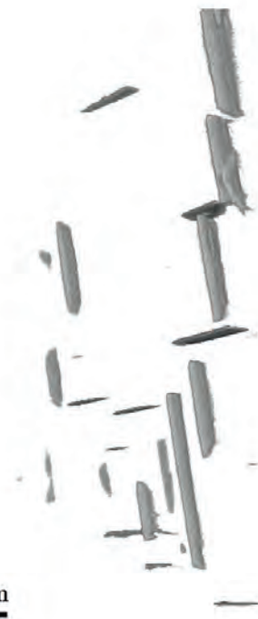
Precipitates, growing along a dislocation line, in an Al-Cu alloy (3D-TEM).
